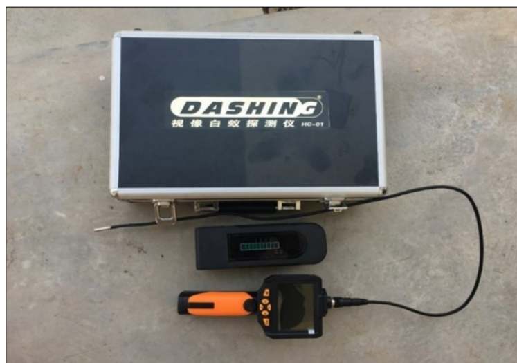
Fig.5. HC-01 visual termite detector fitted with a microwave sounder" used on site
