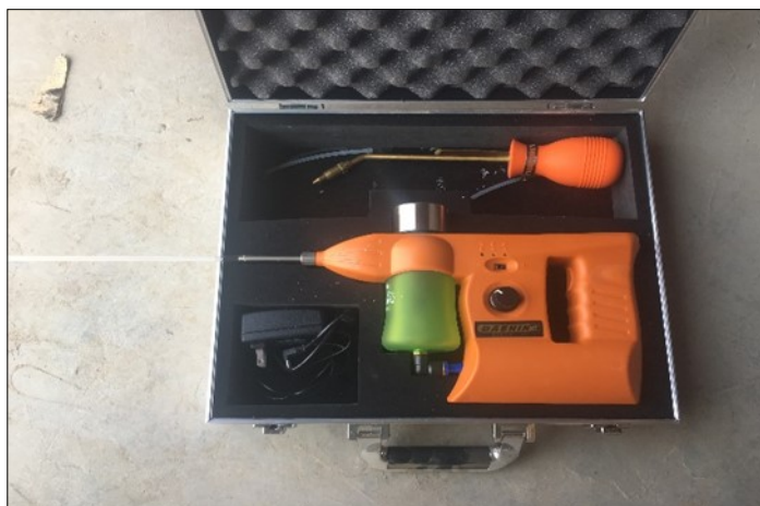
Fig. 7. Duster and shot ball chemical sprayer used at site.
